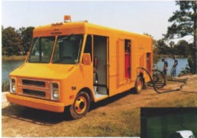
Metito Model CV, complete self-contained mobile chlorination vehicle for emergency or temporary disinfection purposes.
